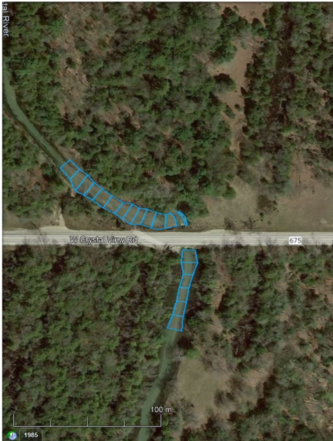
Figure 2. Overview of Crossing 3 with survey cells. Cells are numbered 1 – 19, starting with the northernmost (downstream) cell at top of figure.
